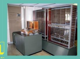
Konrad Zuse develops the first functional digital computer, the ZUSE Z3. It achieves 2 arithmetic operations per second, measured as 2 FLOPS.
